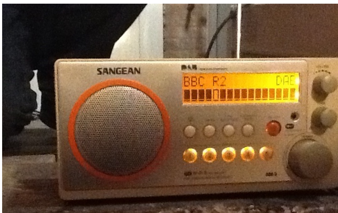
Fig 4: One of the ACI checking receivers showing perfect reception of the BBC multiplex ~7.4 metres away from the transmitting aerial. The BBC transmitter was 3.3 km distant.
