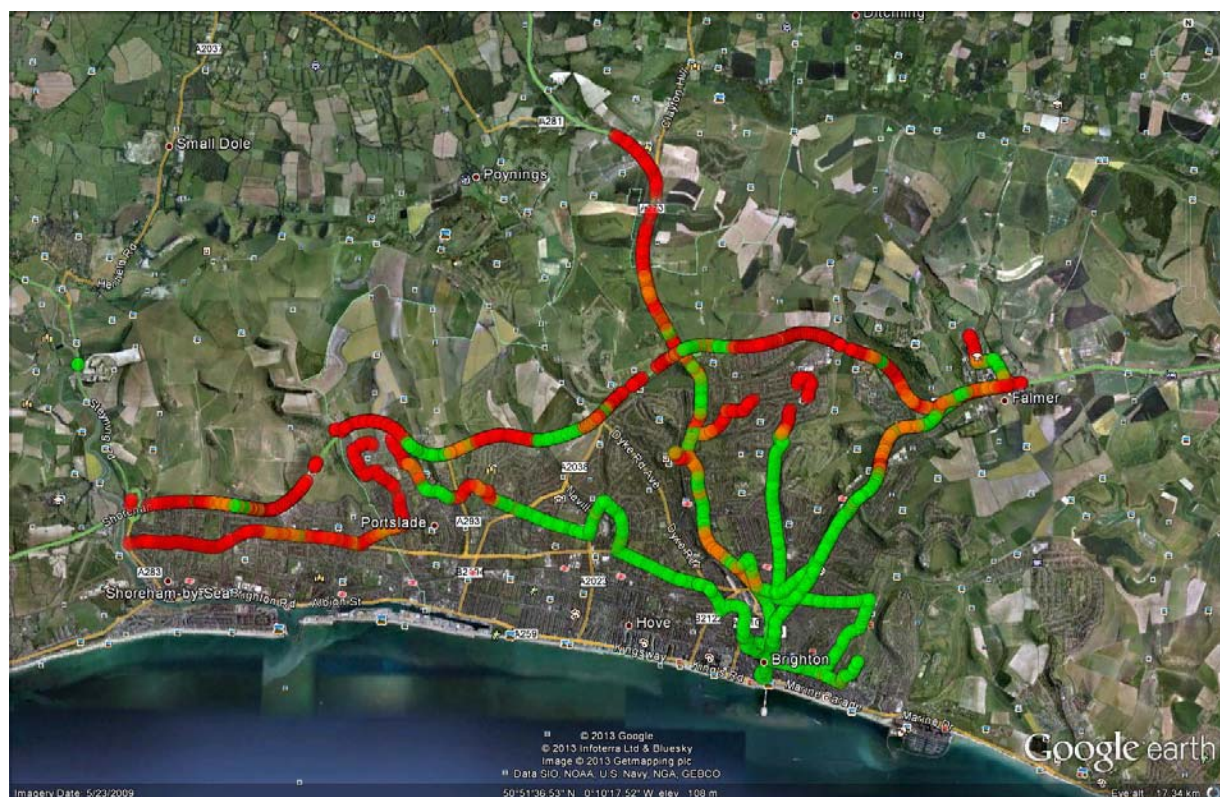
Fig. 8 – Mobile measurement route – reception was available at all logged points. The colours denote the field strength, adjusted to the likely indoor field strength. Green=58dBμV/m, Orange=52dBμV/m, Red=42dBμV/m.
